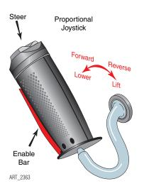
• Function speed is proportional and is controlled by the movement of the joystick.
