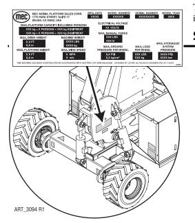
The serial plate is attached to the machine at the time of manufacture. Important information about the machine is recorded on the serial plate.
